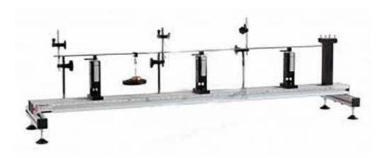
An unlimited range of beam experiments can be conducted to measure support reactions, deflections, and rotations for simply supported beams, fixed beams, two-span continuous beams, simple and propped cantilevers, and sinking supports.
